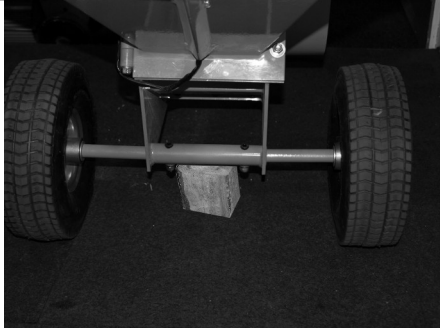
Stage 1 – remove from packing. Support securely and fit the axle.
