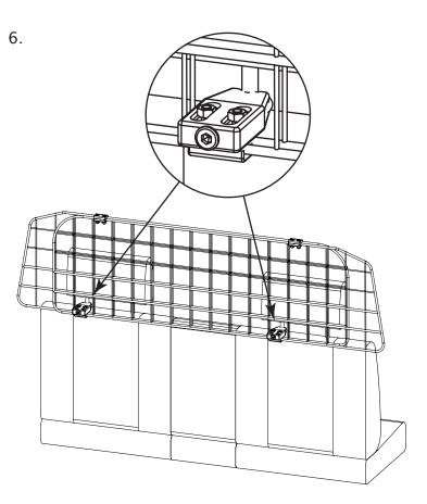
An alternative method of lowering the height if just a small reduction is required, is to mount the headrest clamps upside down, so that the mesh wire is clamped underneath the clamp.
