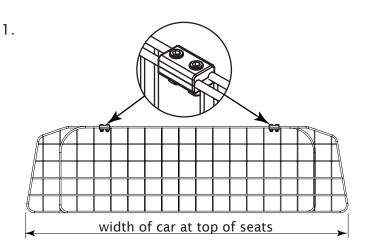
Measure the width of the car at the top of the seat backs. Overlap the two meshes to approximately the measured width, ensuring that the mesh squares align. Clamp the two meshes together at the top using the small clamps. Do not fully tighten the clamps at this point.
