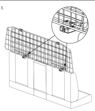
Open the gap between the two meshes at the bottom, so they can fit over the mesh clamps and then slide the mesh into the groves in the clamps.
