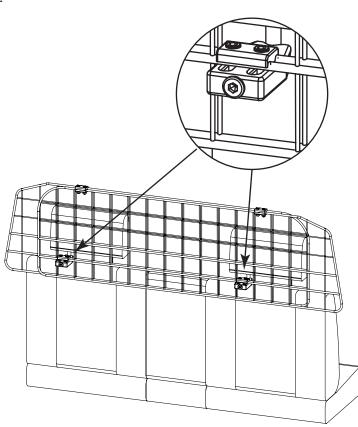
If the mesh is too tall for your car, it can be lowered by using the first or second internal horizontal mesh wires to secure the mesh to the headrest clamps.
