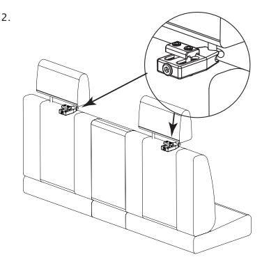
Attach the headrest clamps to one post of each headrest. Which combination of posts you need to use, will depend on how the mesh aligns with the posts. Do not fully tighten the clamps to the posts. The mesh clamp should be sufficiently loose that the mesh can slide underneath.
