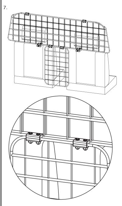
The procedure for mounting the guard to the front seat headrests is exactly the same as for mounting to the rear seat headrests.
