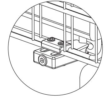
Ensure the mesh is located correctly then tighten the bolts holding the mesh to the clamps and also tighten the clamps to the headrests. Tighten the clamps at the top of the mesh.
