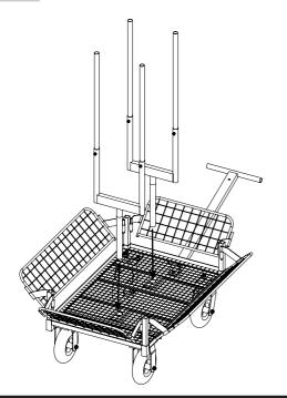
Insert the central support post of a "U Section" into each of the tubes so that it rests on the bolt inserted through the bottom.
