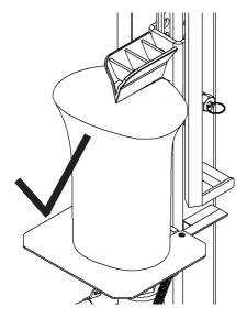
If splitting a log of extremely irregular shape, e.g. where one end flares considerably in diameter. Place the log so the widest end is uppermost.
