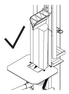
If splitting a log that has already been split, always place the log so the the rounded outer face is against the blade back plates.
