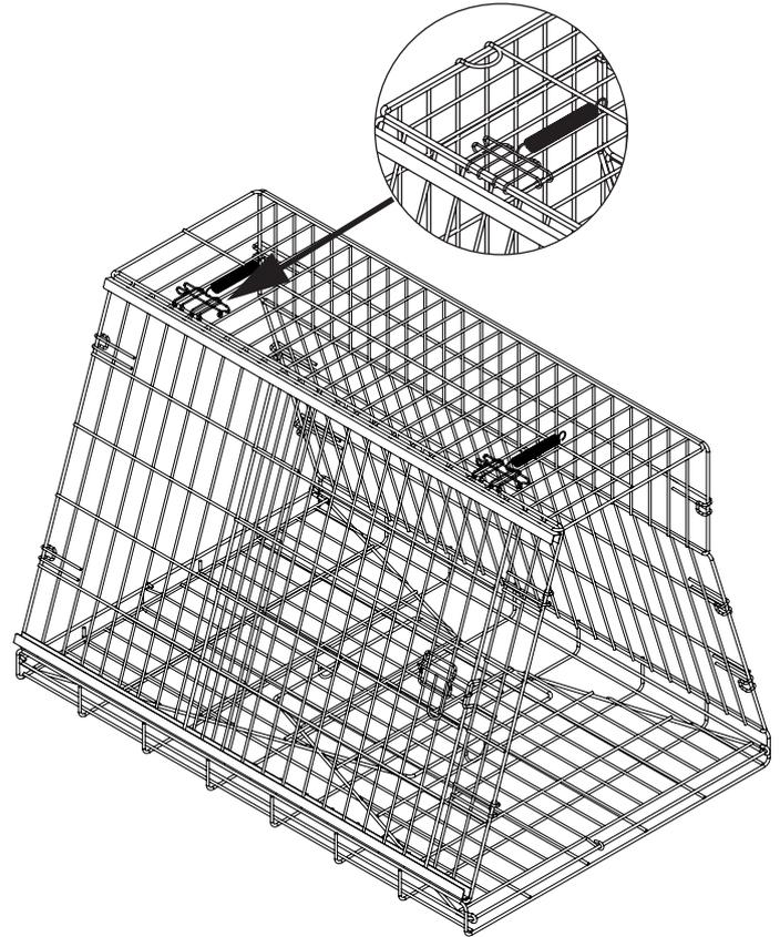
Fold out the top panel and connect to the front with the spring clips
