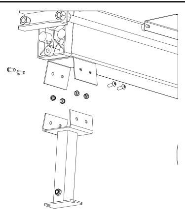
3. Remove the 4 bolts and nuts holding the front leg to the body and remove the front foot assembly from the log splitter. Keep the nuts and bolts as they will be used to attach the stand front leg.
