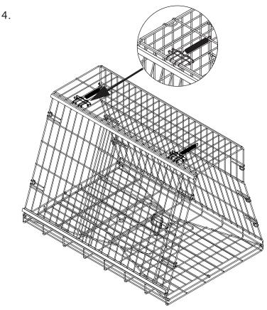
Fold out the top panel and connect to the front with the spring clips
